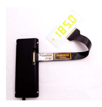
TASEL Introduction Package (TIP) ELT40S is a bundle of one TASEL® display panel (Lumineq ELT40S TASEL display), flexible printed circuit (FPC) cable and driving electronics.
