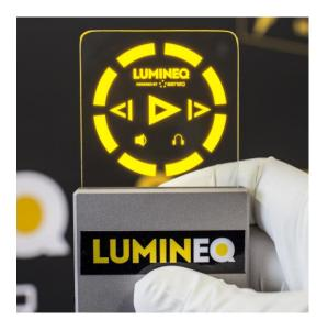
The ELT15S-1500 is a high brightness TASEL<sup>®</sup> transparent segmented display demonstrator that exhibits the full see-through properties of a TASEL display, be that for functional or aesthetic reasons.
