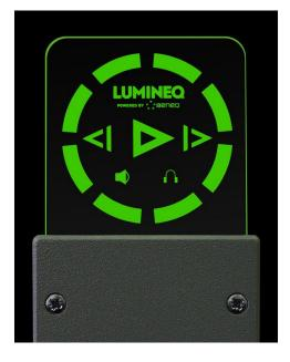
The ELT15S-Green is a TASEL<sup>®</sup> transparent segmented display demonstrator that exhibits the full see-through properties of a TASEL display, be that for functional or aesthetic reasons.
